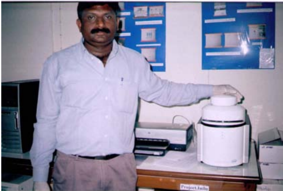
The Real Time PCR employed by Dr.Prakash for viral load assay at NHRBC.
